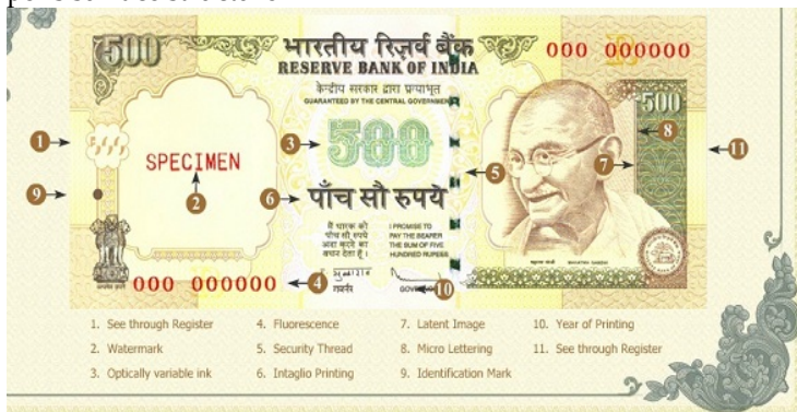
Fig 1: Security Features on Indian Banknote
